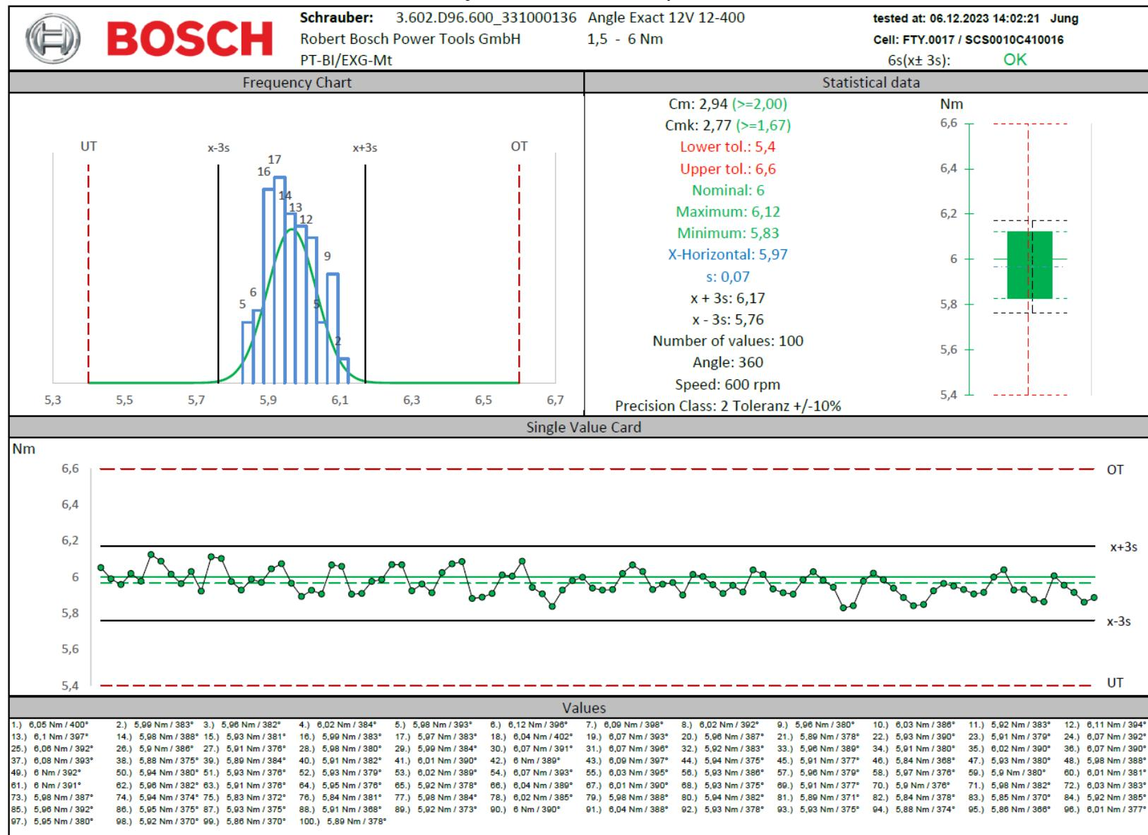
2.1.8.1 Screw joint 360° (soft) Set point 6,0 Nm (100%) 25/100
