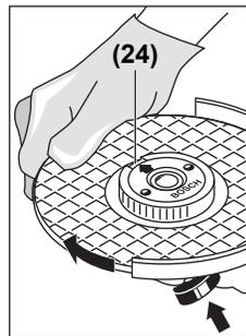
Press the spindle lock button (1) to lock the grinding spindle. To tighten the quick-clamping nut, turn the grinding disc firmly clockwise.
