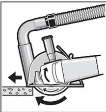
Switch on the power tool and position it with the front part of the guide block on the workpiece. Move the power tool with a moderate feed motion that is suited to the material being machined.
