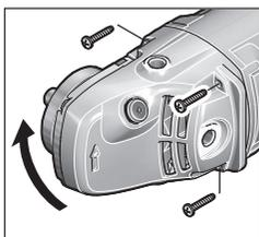
The machine head can be rotated in 90° increments. This enables the on/off switch to be brought into a more convenient position for particular working situations, such as cutting operations using the extraction guard for cutting with a guide block (21) or for left-
