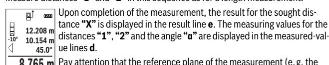
Pay attention that the reference plane of the measurement (e.g. the rear edge of the measuring tool) remains exactly at the same location for all individual measurements within a measuring sequence.
